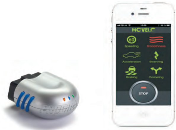
Fig. 1. Examples of measurement probes for insurance telematics: Progressive Insurance Snapshot measurement probe for the OBD outlet (left), (Courtesy: Progressive Insurance); Screenshot of Movelo Smartphone-UBI software RUBI (right) displaying alarm indicators for speeding, non-smooth drives, harsh accelerations, swerving, harsh braking, and heavy cornering (Courtesy: Movelo AB).
